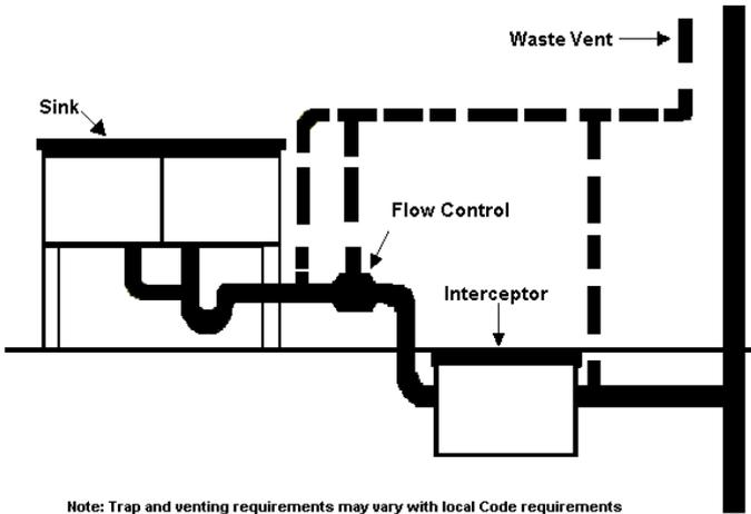
Figure A1.5.7- Interceptor Serving Sink with Flow Control at sink
