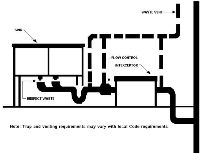
Figure A1.5.13- Interceptor Serving Sinks with Indirect waste
