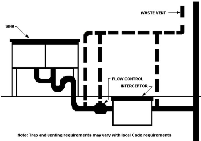
Figure A1.5.6- Interceptor Serving Sink with Flow Control at Interceptor
