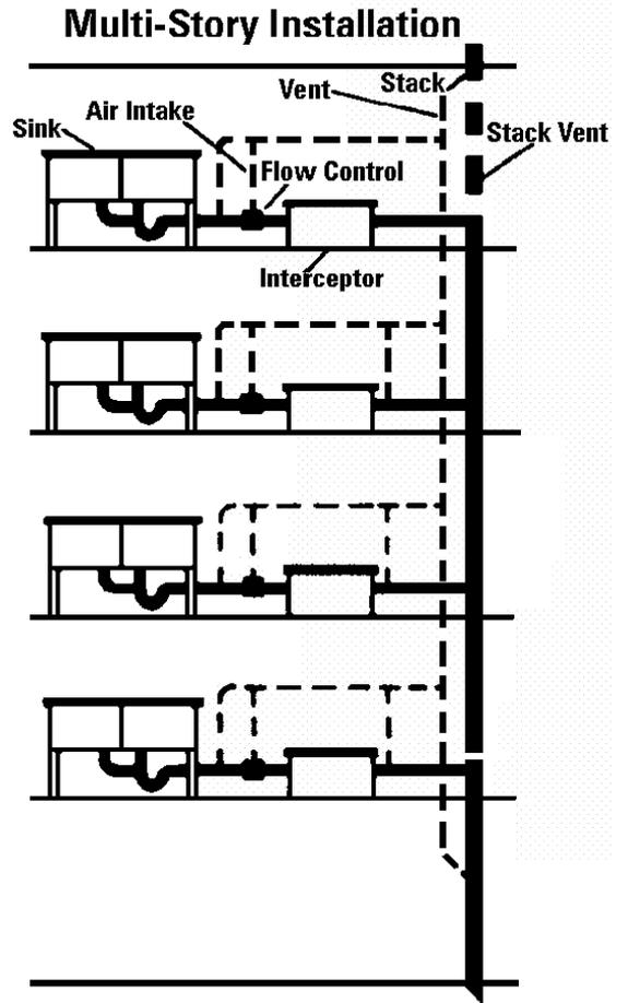
Figure A1.5.5- Interceptors Serving Trapped & Vented Sinks-Flow Control Air Intakes Intersect Vent
